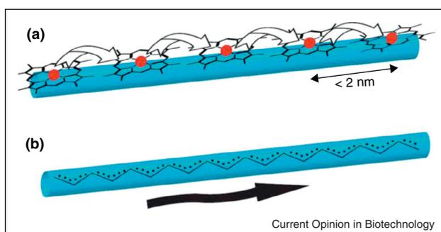
Two contrasting models of electron flow along microbial nanowires. The electron hopping model for filaments of *Shewanella oneidensis* (a) and the metallic-like conduction for pili of *Geobacter sulfurreducens* (b). In the electron hopping mechanism, charges hop from cytochrome to cytochrome (shown in red). In metallic-like conduction, delocalized charges (shown as black dots) are spread across the entire filament.
